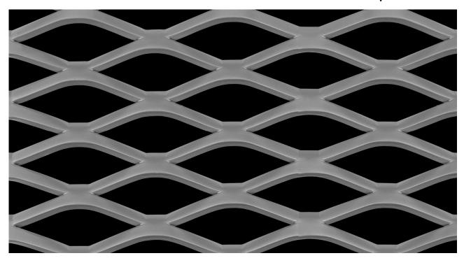
LW Pitch:60.96mmStrand Width:6.00mmSW Pitch:25.00mmThickness:4.00mmWeight:15.07 kg / m2 (Black Weight)Open Area:52%
